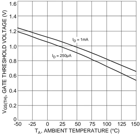
Fig. 7 Gate Threshold Variation vs. Ambient Temperature
