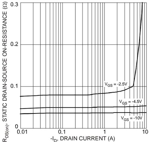
Fig. 3 On-Resistance vs. Drain Current and Gate Voltage
